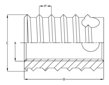
Female thread A = M12 Length B = 12 Male thread E = 16.0 Min hole depth blind hole = 15 Thread pitch P = 1.75
